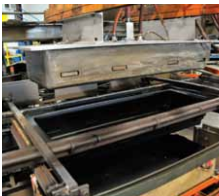
Vacuum mold for keyboard case
