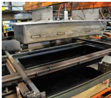
Vacuum mold for keyboard case
